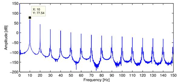
Figure 4. Output spectrum of the high voltage power supply when driven with a 10 Hz modulation of approximately 250 V<sub>PP</sub> added to a DC level of 1500 V. The waveforms were acquired from the feedback output of the supply. Notice the apparent nonlinear distortion.
