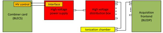
Figure 3. Simplified view of the modulation signal chain.
