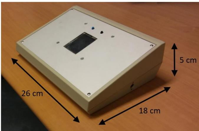
Fig. 1. The developed measurement device and its dimensions.
