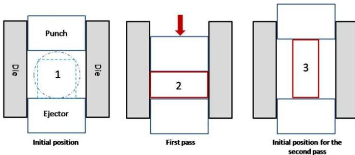
Figure 2 Schematic closed die forging
