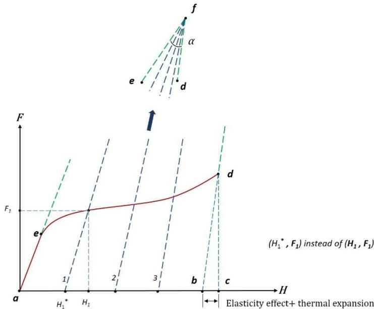
Figure 3 The method of force-height data correction
