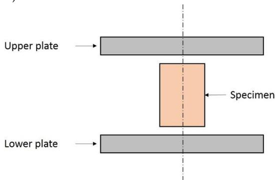
**Figure 1** Schematic of open die forging
