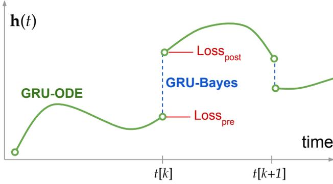
Fig. 1. GRU-ODE-Bayes uses GRU-ODE to evolve the hidden state between two observation times  $t[k]$  and  $t[k+1]$ . GRU-Bayes processes the observations and updates the hidden vector  $\mathbf{h}$  in a discrete fashion, reflecting the additional information brought in by the observed data.
