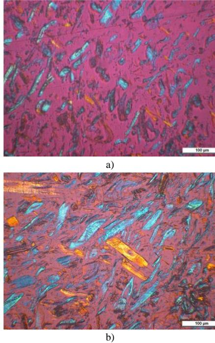
**Fig. 2** POM micrograph recorded on W126 composites; a) 20, b) 40 vol% wood. Development of a fiber network at large wood content.
