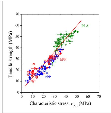
**Fig. 3** Close correlation between the initiation stress of the dominating deformation process and the strength of the composite. Symbols: PLA: ●●●●●●, rPP: ▲▲▲▲▲▲, hPP: ■■■■■■, CC23: ●●●●●●, W35: ▲▲▲▲▲▲, W54: ●●●●●●, W68: ▲▲▲▲▲▲, W125: ●●●●●●
