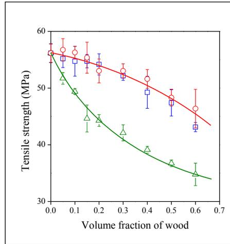
**Fig. 1** Effect of wood content and coupling on the tensile strength of PLA/wood composites; Symbols:  $\square$  BMI,  $\circ$  DBMI,  $\triangle$  no coupling.
