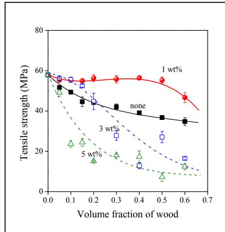
**Fig. 4** Dependence of the tensile strength of PLA/wood composites on wood content and on the concentration of the resin solution used for impregnation. Symbols: ■ neat, ● 1, □ 3, △ 5 wt% resin solution.
