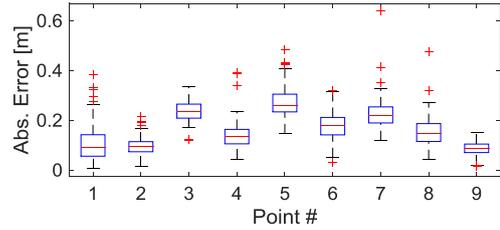
Fig. 5. Boxplot representation of the positioning error over the repeated measurements represented in Fig. 3. The central line of each box is the median error while the edges of each box represent the first and third quartile. Top and bottom ends of the dashed black lines are the maximum and minimum error with the red plus symbols representing outliers.
