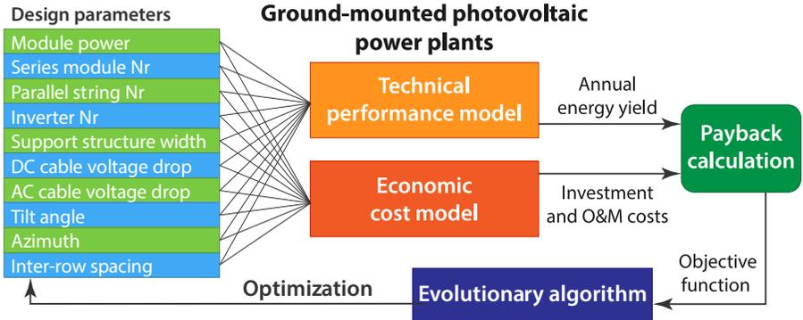
**Fig. 2** Concept of the design optimization of ground-mounted PV plants for the financial payback
