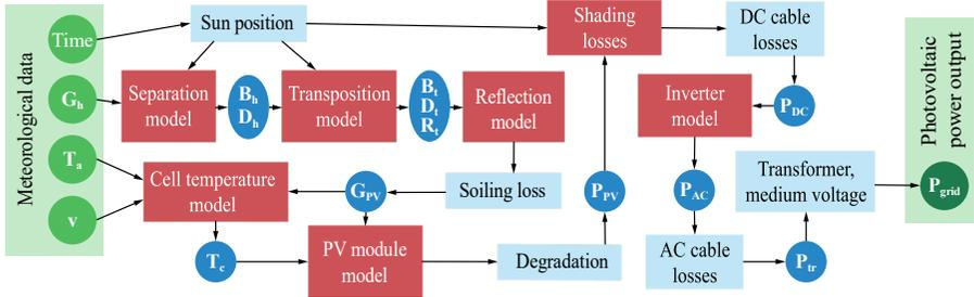
**Fig. 1** Concept of the physical PV performance modeling based on weather data. Red boxes indicate the seven main modeling steps where multiple model variants are compared
