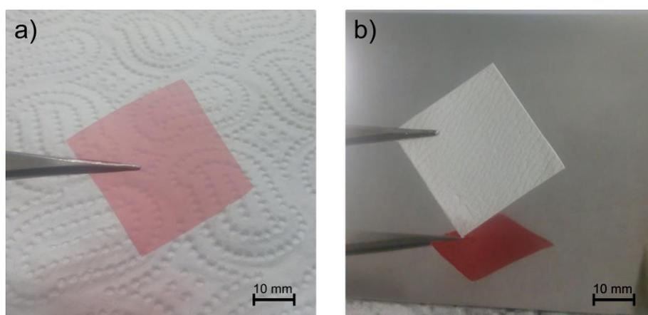
**Figure 3. (a) Casted and cut (30 × 30 mm) pullulan film with incorporated citric acid and (b) the final ODW with the nanofibrous layer containing 6.25 mg CAR.**
