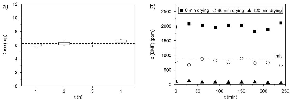
**Figure 4.** (a) The results of content uniformity measurements of the ODW products prepared using the continuous system in steady state and (b) residual DMF content of the final product during 4-hour long operations of the continuous system at different drying times.
