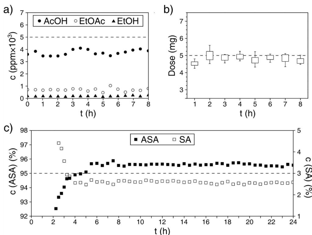
**Figure 2. Quality attributes of ODWs over time produced by the CMS: (a) residual solvent content, (b) content uniformity, (c) and purity (HPLC). The dashed lines indicate either regulatory (residual solvent) or specified process (minimal accepted ASA purity and target dose) limits.**
