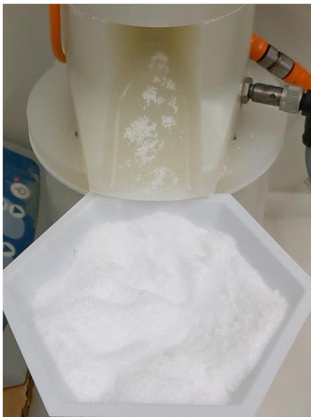
**Figure 5. Dry, free-flowing ASA crystals from the integrated continuous crystallization-filtration experiments.**
