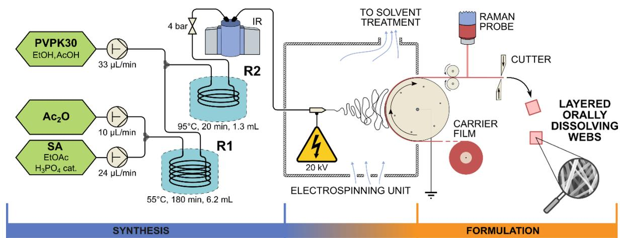
Figure 1. Schematic diagram of the developed system for the production of ASA-loaded fibrous ODWs based on ES. R1 and R2 microreactors, IR Bruker FTIR cell, Kaiser Raman PhAT probe.
