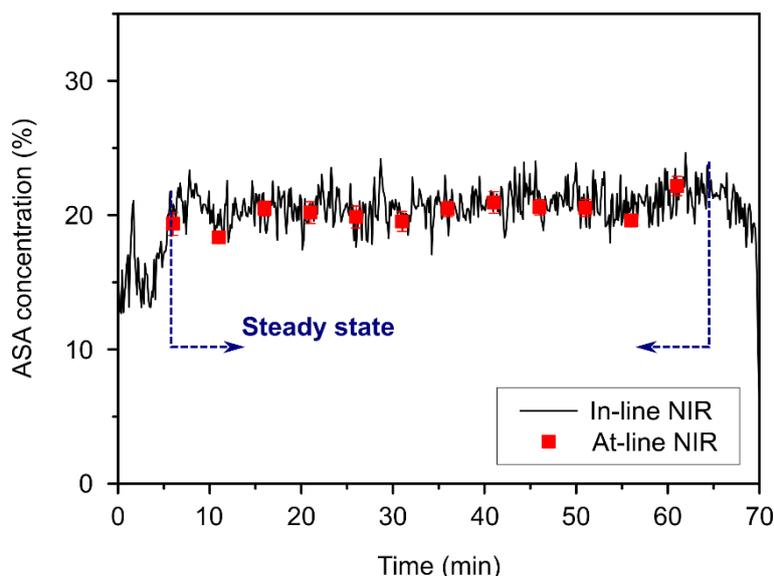
**Figure 6. ASA concentration in the powder blend measured by an in-line NIR probe after blending, and the result of at-line NIR analysis of the produced tablets from the steady state.**
