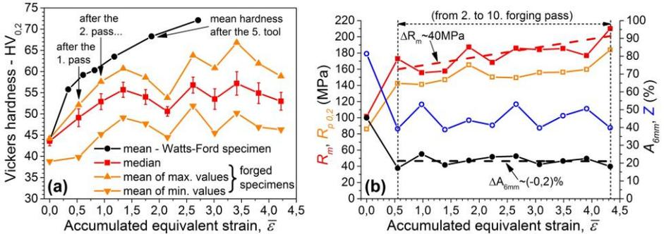
**Figure 4** The evolution of (a) the hardness and (b) the mechanical properties of EN AW-6082 aluminum alloy during multi-axial forging
