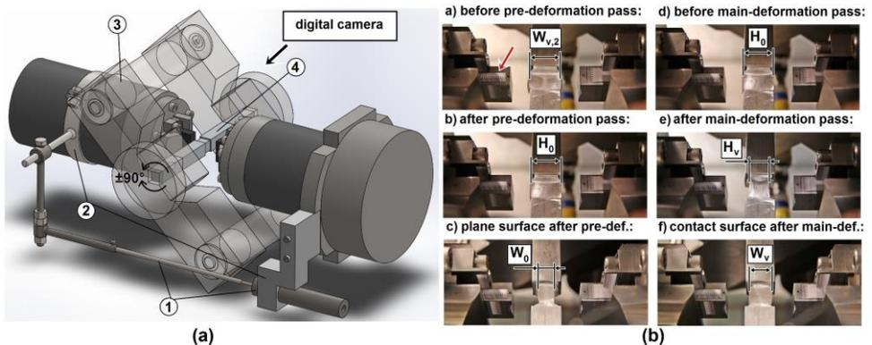
**Figure 1** (a) The 3D model of the functional parts of the MaxStrain device
