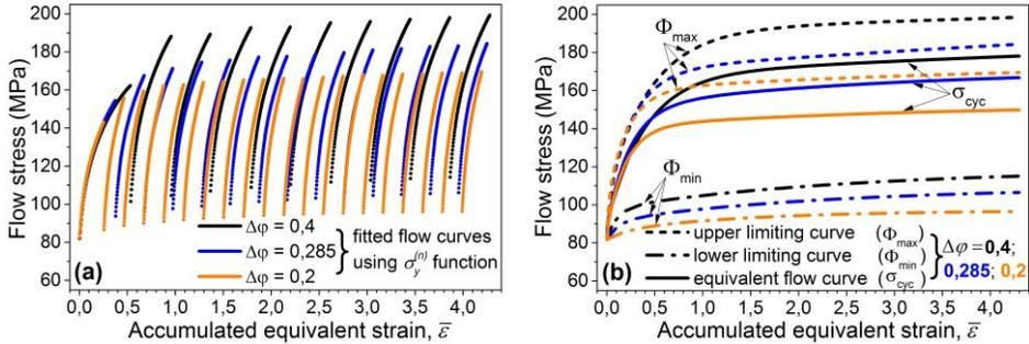
**Figure 3** (a) The fitted flow curves which describes the evolution of flow stress under multiple forging with different strain amplitudes and (b) the limiting as well as the equivalent flow curves of the flow stress
