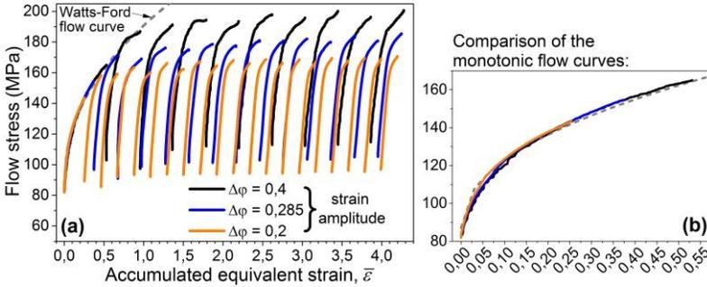
**Figure 2** (a) The flow curves of the multiple forging simulations with different strain amplitudes and (b) the enlarged flow curves for the first pass
