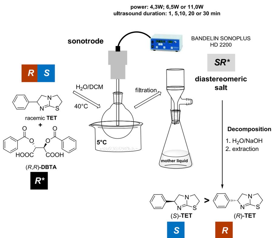
Figure 6. Schematic figure of ultrasound-assisted resolutions
