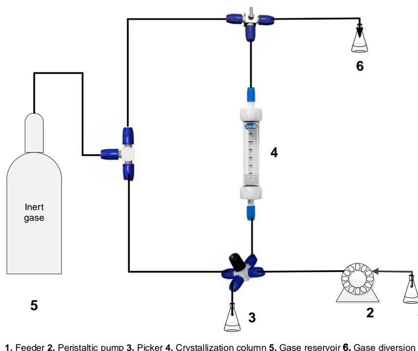
**Figure 9. Scheme of appliance for method named „resolving agent in a cage”**
