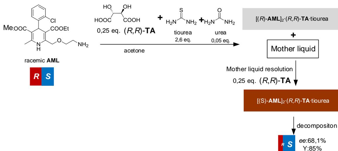
**Figure 5. Diastereomeric salt resolution of amlodipine**
