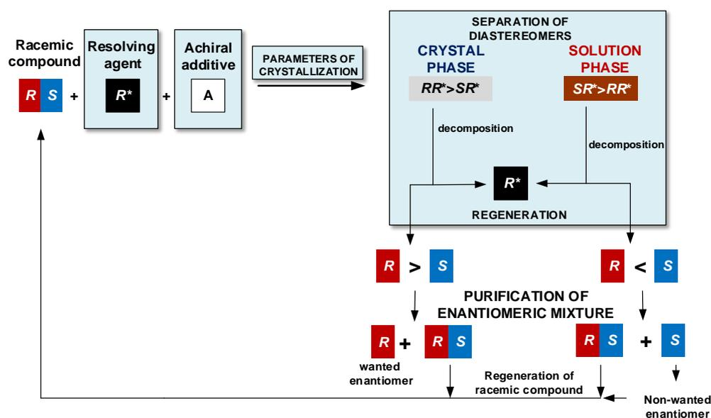
Figure 1. Route to the pure enantiomers via diastereomeric salt resolution
