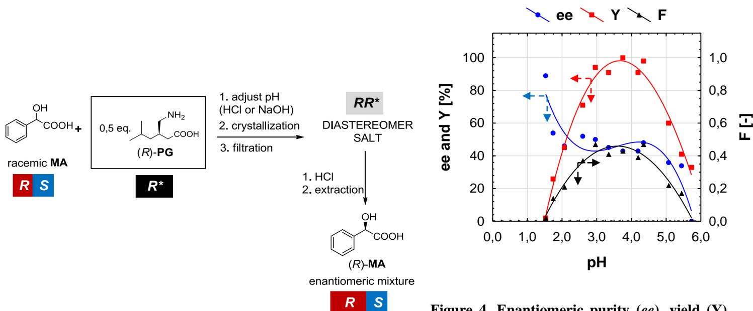
Figure 3. pH-dependency of the MA resolution with (*R*)-PG
