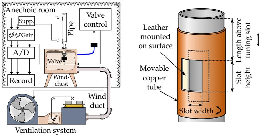
Figure 3. Sound spectrum measurement setup (left), adjustable tuning slot (right)
