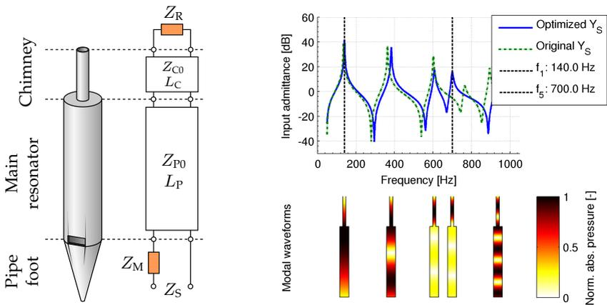
**Figure 1.** Chimney pipe model (left) and admittance optimization (right)
