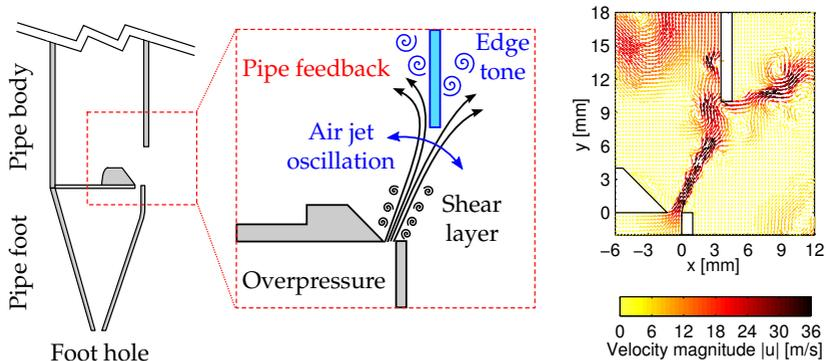
**Figure 6.** Pipe foot model (left) and edge tone simulation (right)
