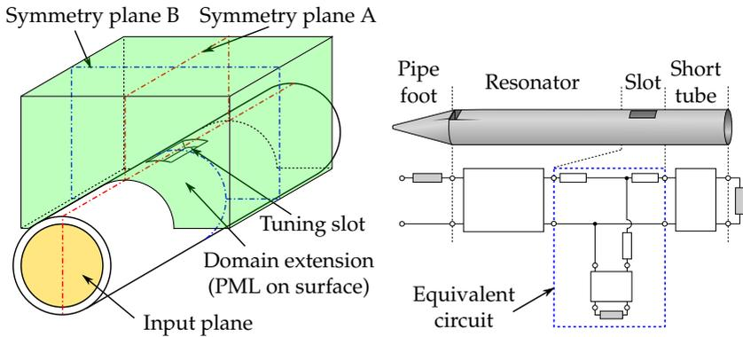
**Figure 4.** FE / PML tuning slot model (left) and its equivalent circuit (right)
