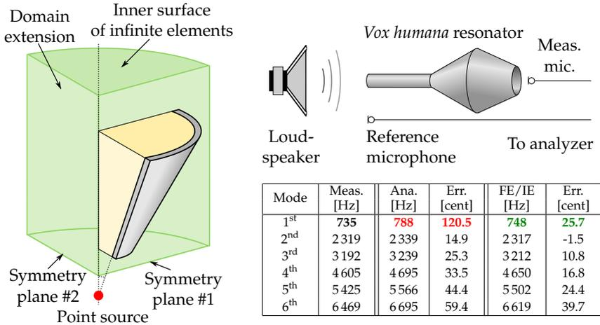
**Figure 5.** Radiation impedance model (left) and its application (right)
