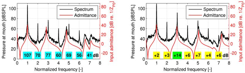
**Figure 2.** Chimney pipe optimization: original pipe (left), optimized pipe (right)
