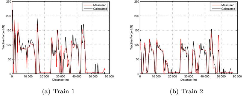
Figure 3: Measured and calculated traction forces
