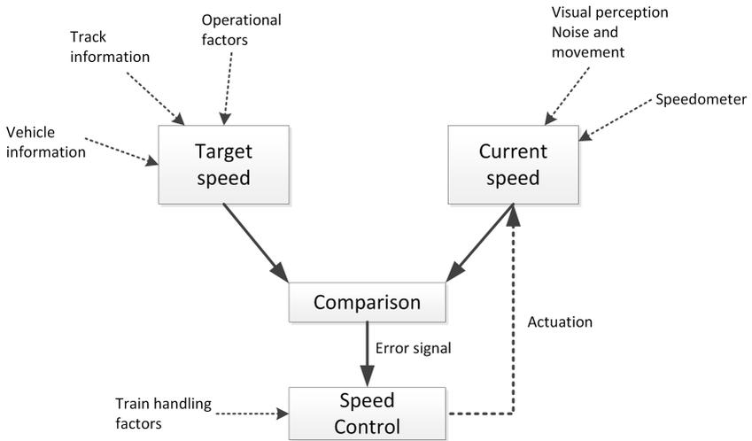
Figure 1: Human speed control process
