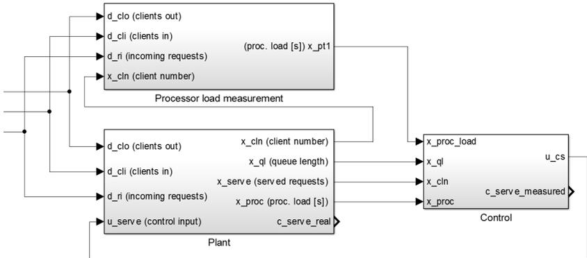
Figure 2: Schematics of the control architecture
