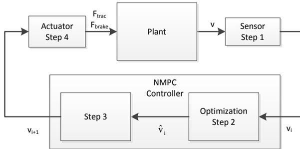
Figure 5: The control loop
