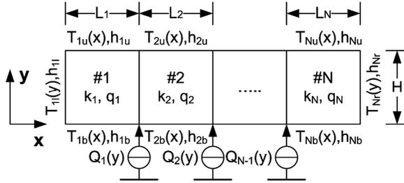
**Fig. 3: The model of the multilayered medium.**
