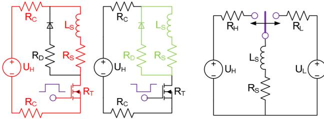
**Fig. 2: Non-ideal PWM drive configuration and its generalization.**
