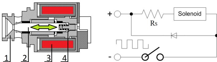
**Fig. 1: Structure of an electromagnetic valve (left side) and PWM drive (right side): 1-valve, 2-spool, 3-electric coil, 4-return spring.**
