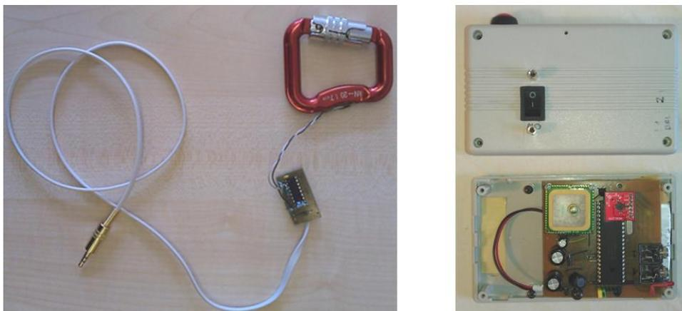
**Figure 3:** Force sensor developed (left) and the data acquisition system (right)
