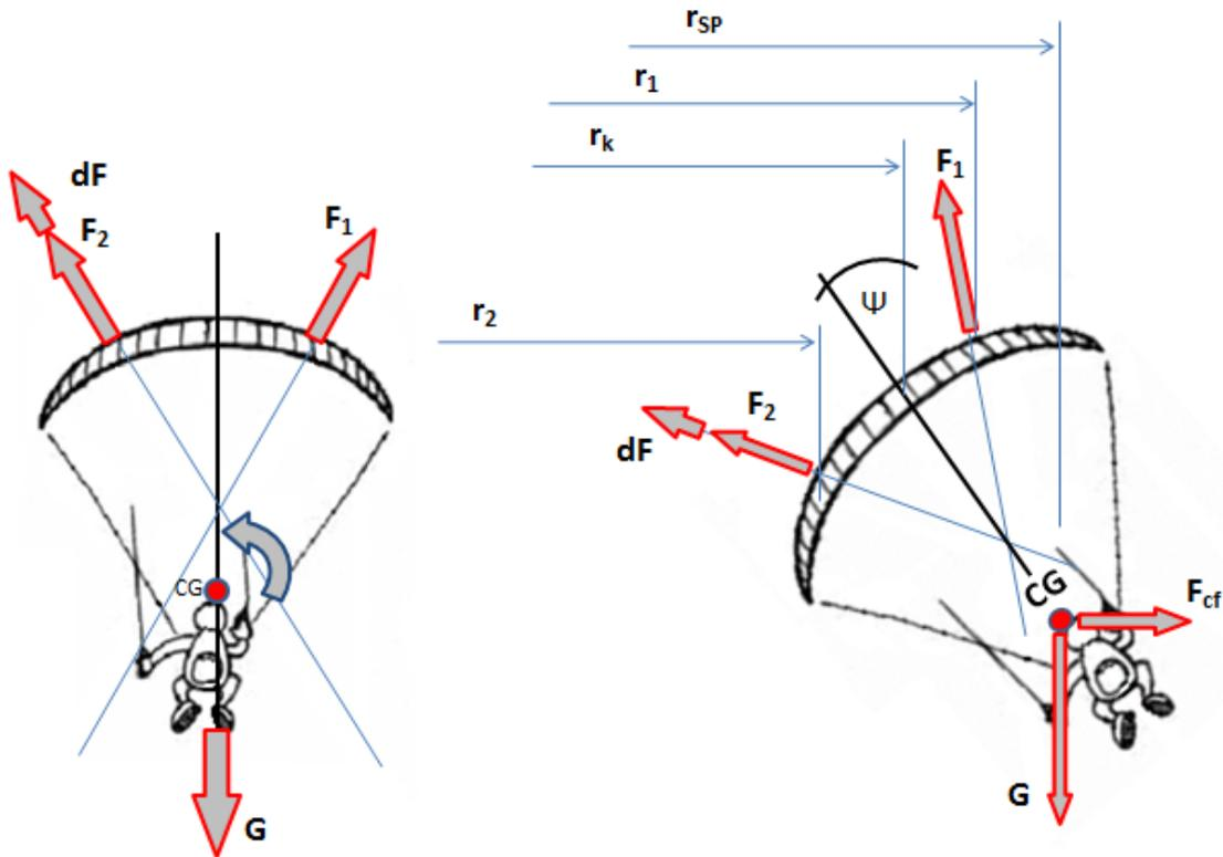
**Figure 2:** Considered forces on a paraglider in static, balanced turn
