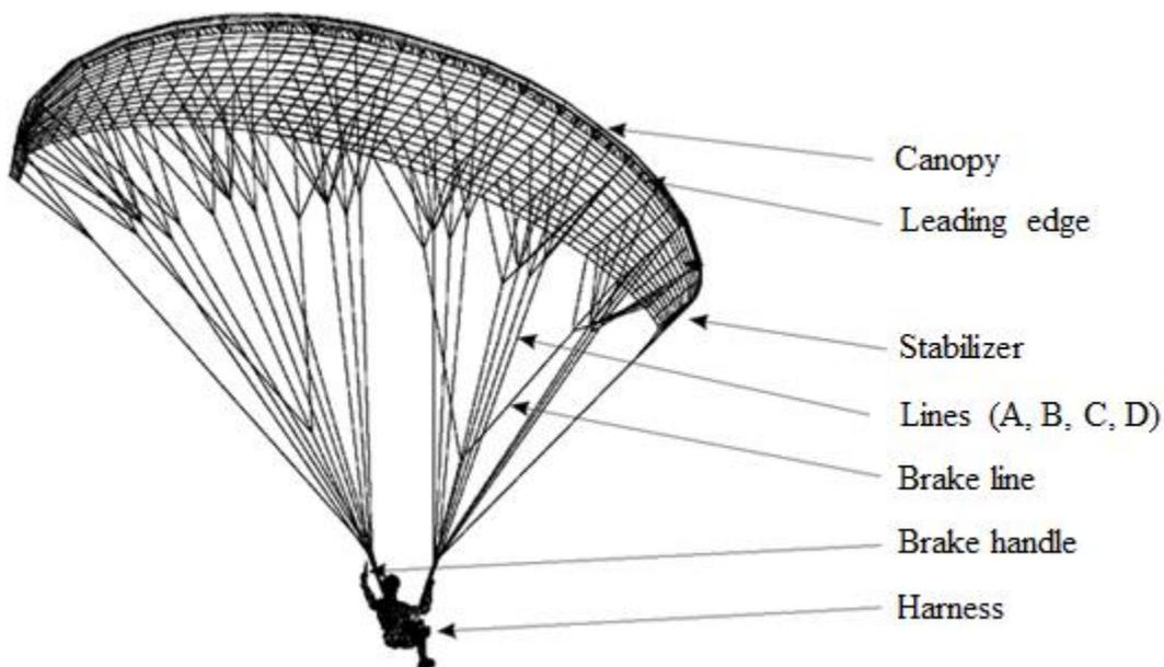
**Figure 1:** The general structure of a paraglider
