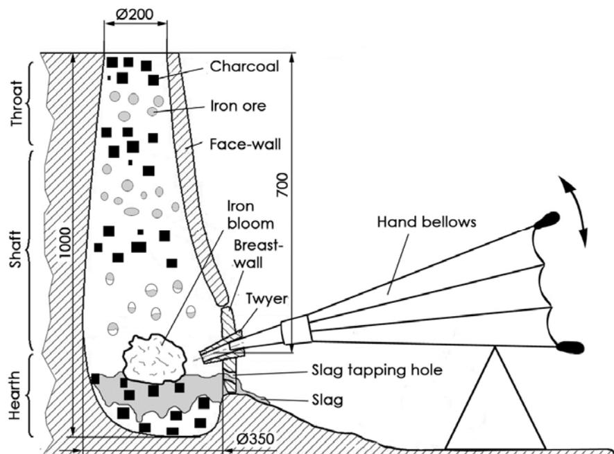
Figure 1: Fajszi-type furnace used in the smelting experiments and the terminology
