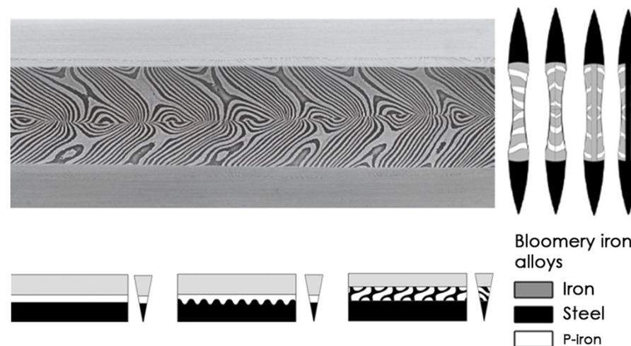
Figure 2: Pattern welded sword blades (6-10th century) and knife blades (9-15th century) decorated with phosphoric iron layers.
