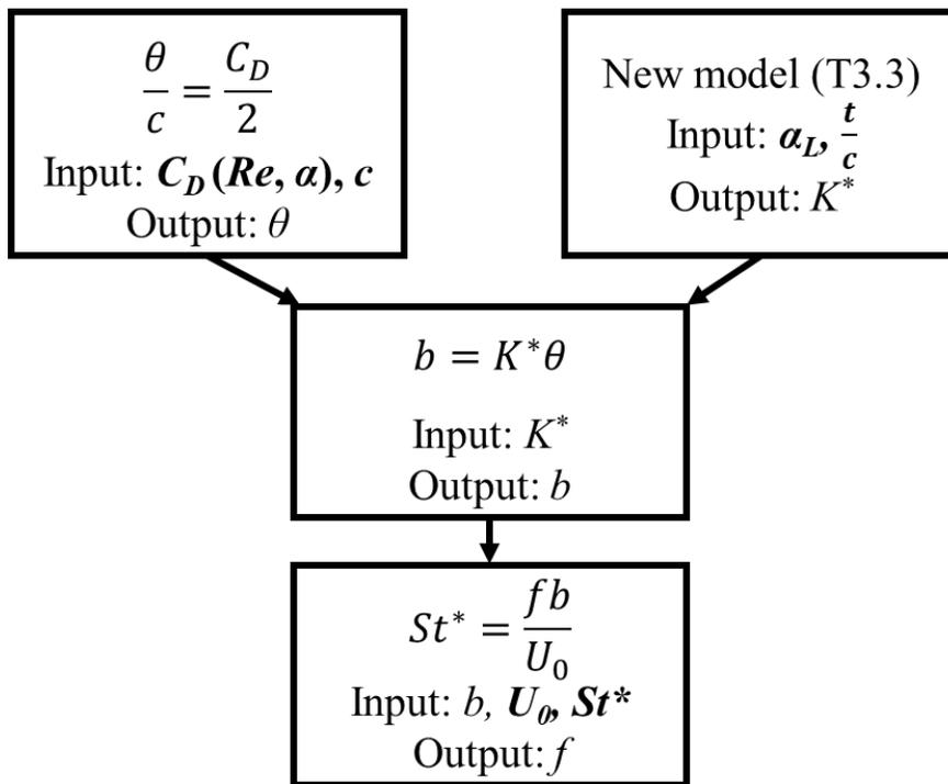
Figure T 3.2 Flowchart presenting the process of profile vortex shedding frequency estimation.
