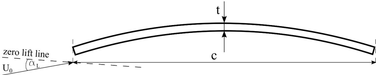
Figure T 3.1 Sketch of a profile with indication of characteristic quantities
