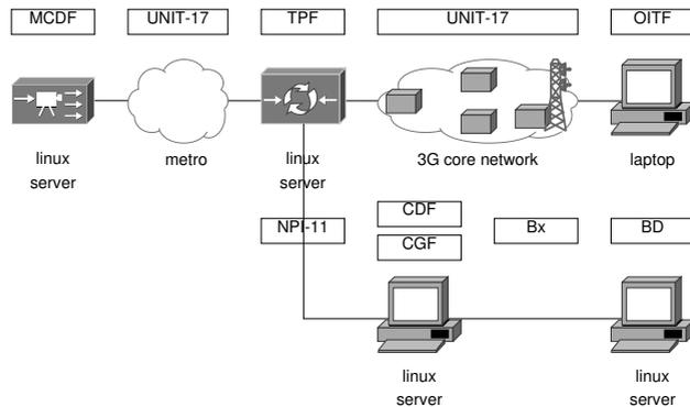
Figure 2. Testbed for quality based charging simulation
