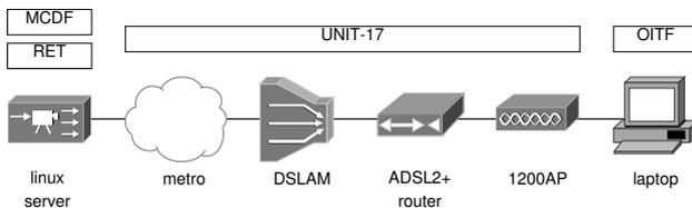
Figure 1. Testbed for IPTV retransmission simulation
