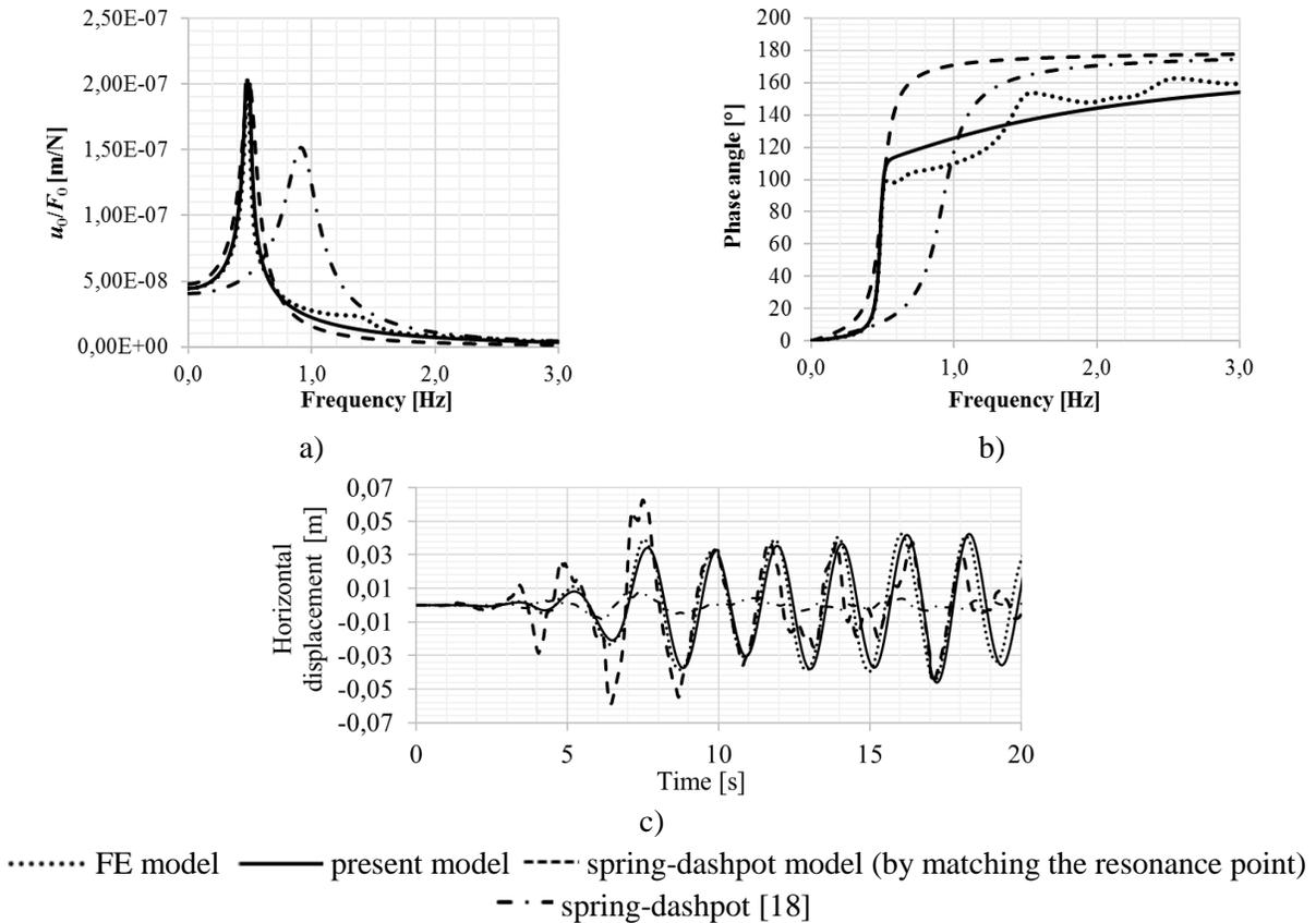
**Fig. 6** a) amplitude, b) phase angle of the impedance function with damping, c) solution of the different models for an earthquake record ([17] record no. 32)
