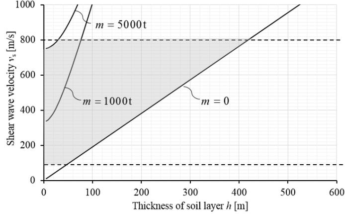
**Fig. 4** Parameter range ( $v_s$  and  $h$ ), where the natural frequency of the system is in the range of the dominant frequency of earthquakes
