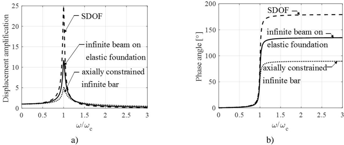
**Fig. 2** Amplification factor (a) and phase angle (b) of the SDOF system, axially constrained infinite bar and beam on elastic foundation with damping,  $\zeta=2\%$
