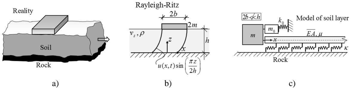
**Fig. 5** Simplified models of a soil layer with an object, a) reality, b) 2D model, c) 1D model
