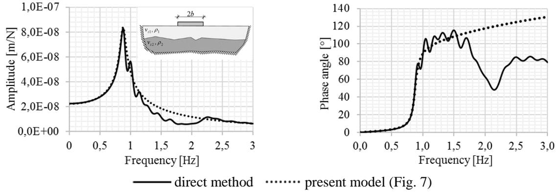
**Fig. 10** Impedance curves for irregular soil layers ( $v_{s1}=100$  m/s,  $\rho_1=1800$  kg/m<sup>3</sup>,  $v_{s2}=250$  m/s,  $\rho_2=1950$  kg/m<sup>3</sup>)
