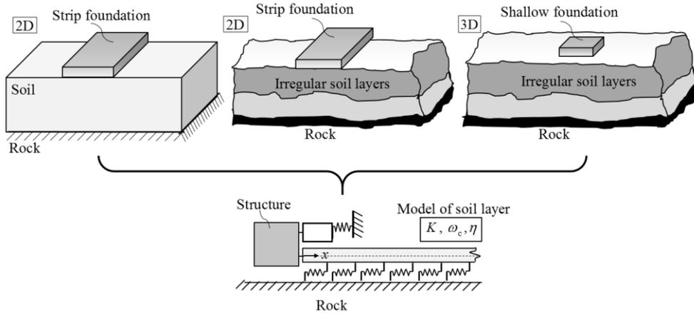
**Fig. 7** Examples of 2D and 3D problems, and the model (the model parameters are:  $K$ ,  $\omega_c$ ,  $\eta$ )
