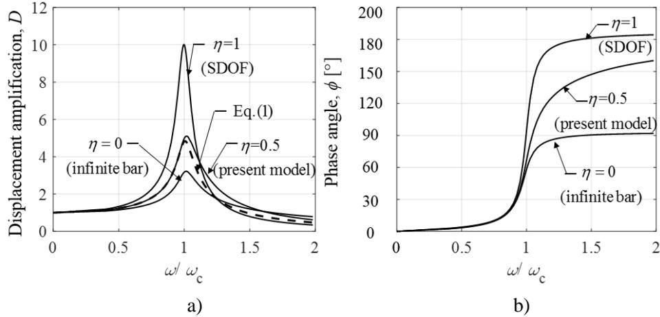
**Fig. 8** Amplification factor and phase angle for  $\zeta=0.05$  damping ratio
