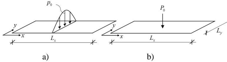
**Fig. 11** Long plate subjected to a trigonometrical line load (a) and to a concentrated load (b)
