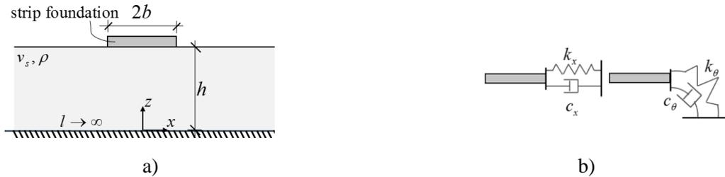
**Fig. 3** a) Finite soil layer with thickness  $h$  and rigid foundation, b) simplified model with constant spring stiffness and dashpot element
