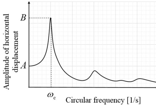
**Fig. 9** Three representative parameters of the impedance curve
