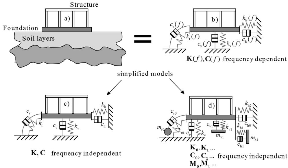
**Fig. 1** The modelling levels of soil effect: a) direct approach, b) impedance function, c) one, frequency independent spring and dashpot element for all directions, d) more complex lumped models
