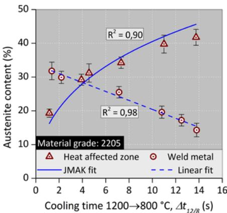
Figure 9. The change of the austenite content in the heat affected zone and in the weld metal as a function of the  $\Delta t_{12/8}$  cooling time for 2205 grade. For the other material grades the relationships can be found in the dissertation.
