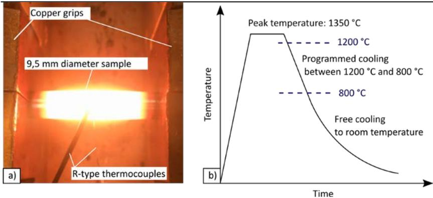
Figure 3. The Gleeble physical simulator setup a) and the schematic representation of the applied thermal cycle b).
