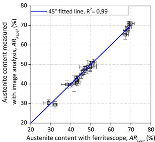
*Figure 1. The results of austenite content measured with image analysis, after optimal etching cycle ( $AR_{Képel}$ ), compared to the austenite contents measured by ferritescope ( $AR_{Ferit}$ ).*
