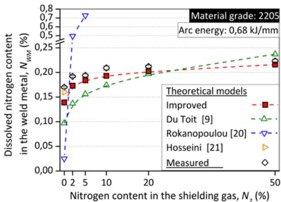
Figure 6. The comparison of my improved model and the previous models [9, 20, 21] for the calculation of weld metal nitrogen content.
