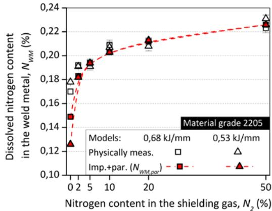
Figure 7. The weld metal nitrogen contents calculated by the parameter-supplemented and improved model ( $N_{WM,par}$ ), compared to the measured ( $N_{WM}$ ) values.
