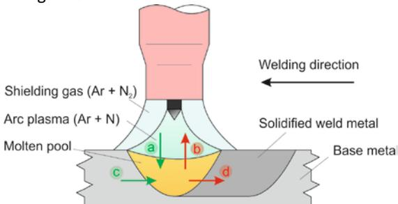
Figure 5. Schematic illustration of the nitrogen absorption: (a,c), and desorption: (b,d) during autogenous tungsten inert gas (TIG) welding of DSS.
