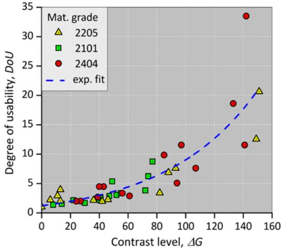
Figure 2. The DoU (degree of usability) number as a function of  $\Delta G$  contrast levels, using Beraha-II type etchant.
