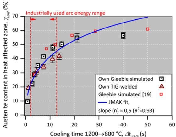
Figure 4. The fitted JMAK equation for the determination of the austenite content of the heat affected zone based on own and ref. [19] results for duplex stainless steel grade 2205.
