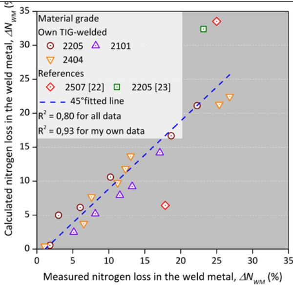
Figure 8. Comparison of the relative reduction in nitrogen content of the welded metal, calculated according to the defined equation, supplemented with literature data [22, 23].
