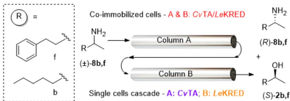
**Figure 5.** Continuous-flow conversion of a racemic amine [(±)-**8b,f**] to enantiopure amine (*R*)-**8b,f** and alcohol (*S*)-**2b,f** performed by a two column-single cell serial cascade or a co-immobilized whole-cells system.
