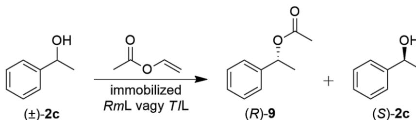
**Figure 7.** Kinetic resolution of racemic 1-phenylethanol ( $\pm$ )-**2c** with immobilized *RmL* or *TIL*
