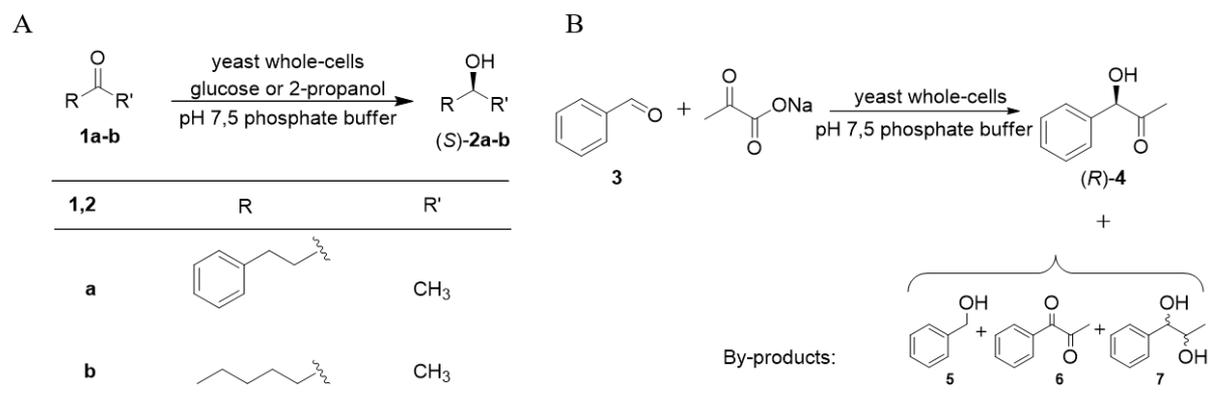
**Figure 1.** Yeast mediated bioreductions (Panel A) of prochiral ketones **1a-b** and acyloin condensation (Panel B) of benzaldehyde **3**.
