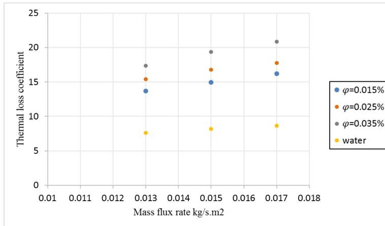
Figure (4): Thermal loss coefficient against the mass flux rate for water and nanofluids for evacuated solar collector
