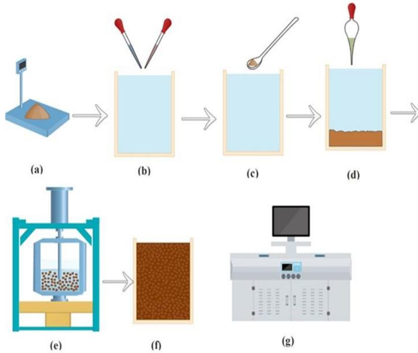
Figure (1): Layout of the synthesis and stability check of nanofluids
