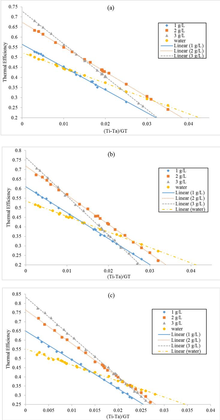
Figure (5): Thermal efficiency of the collector for copper/water nanofluid for evacuated solar collector at different volume flow rate (a) 0.6 L/min, (b) 0.7 L/min, (c) 0.8 L/min
