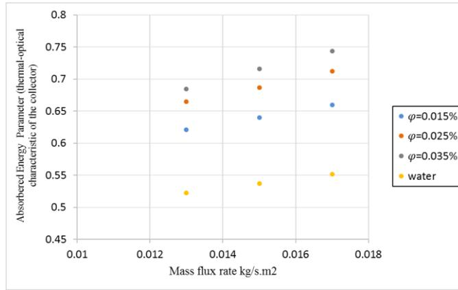
Figure (3): Absorbed Energy Parameter against mass flux rate for water and nanofluids for evacuated solar collector
