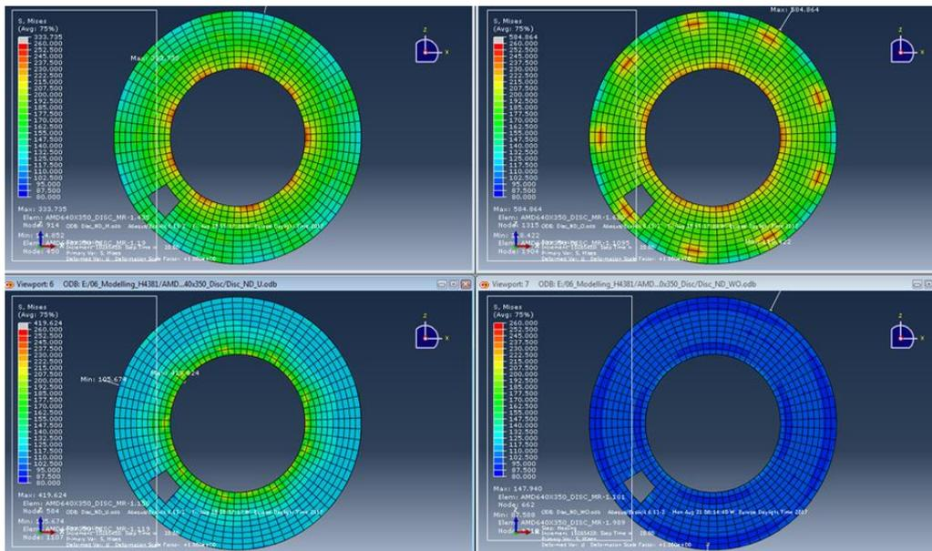
**figure 7: the v. Mises stresses at the friction surface [17]**
