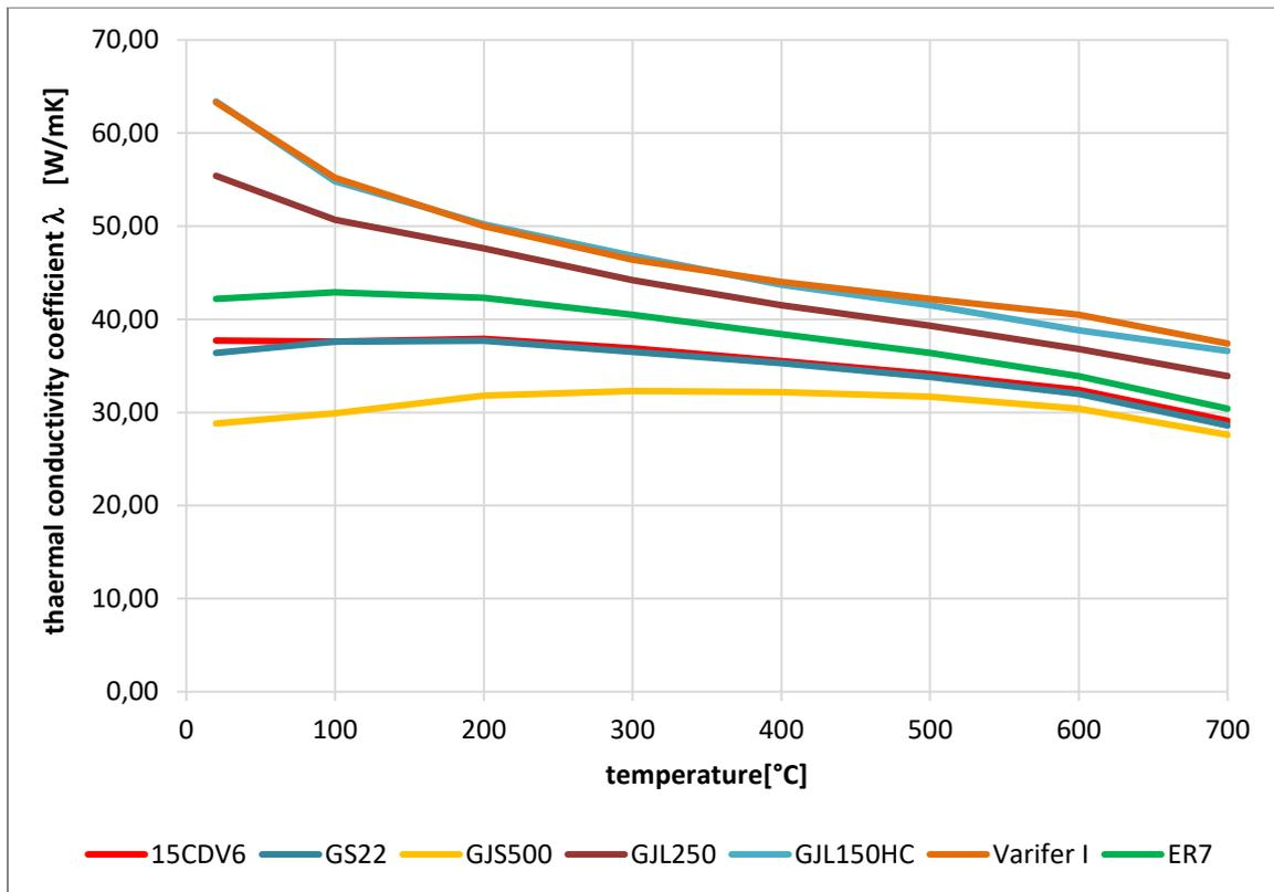
**figure 3: the thermal conductivity coefficient -  $\lambda$  [15],[20]**
