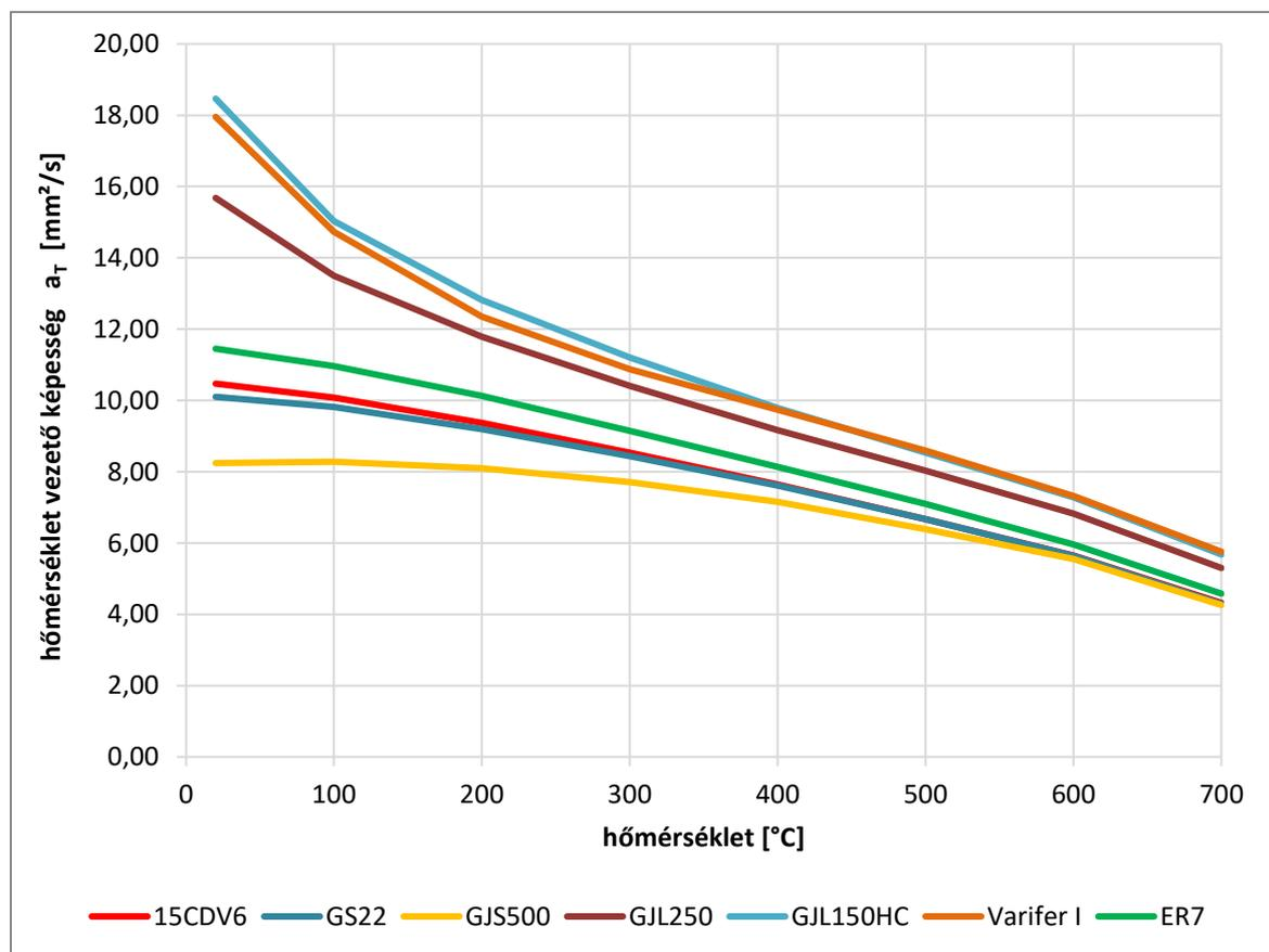
figure 2: the temperature conductivity coefficient  $\alpha_t$  [15],[20]
