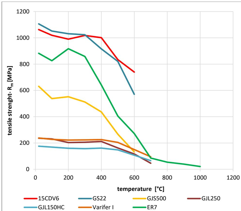
**figure 4: the tensile strength - R<sub>m</sub> [15],[20]**
