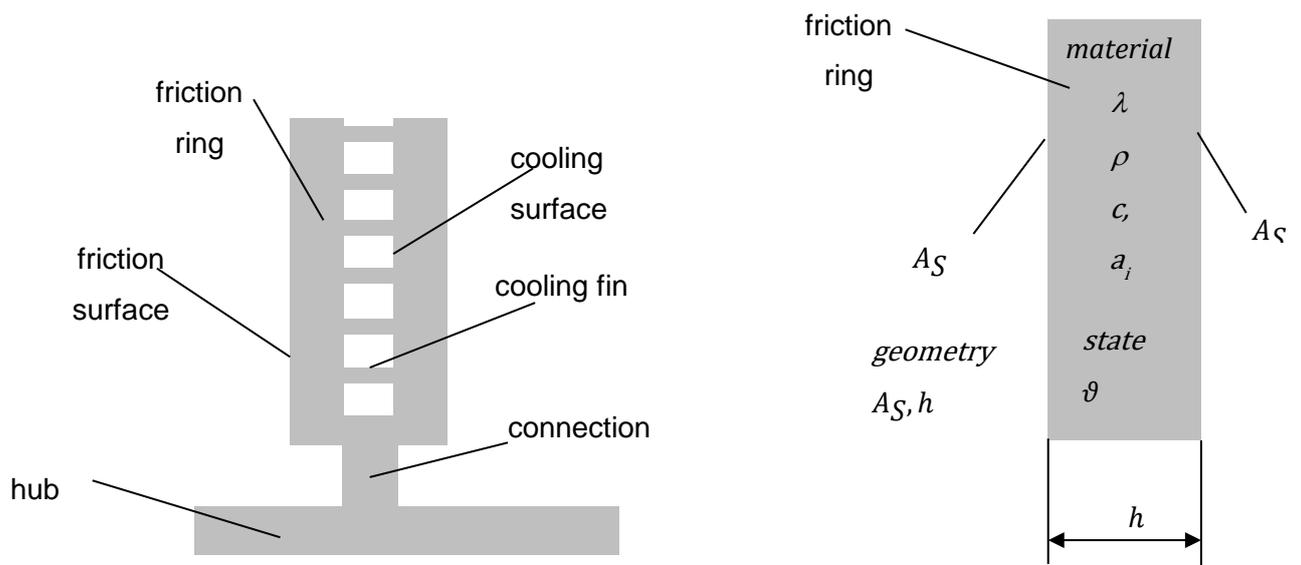
**figure 1 1: Brake disc lower part: Properties of the friction ring**
