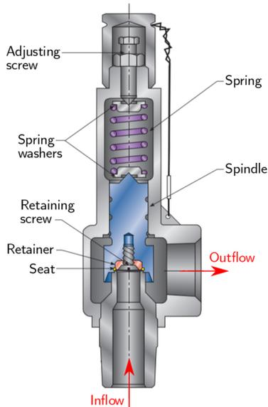
Figure 1.1: A typical direct spring operated valve [2].
