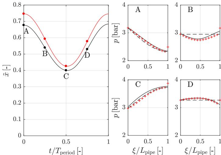
Figure 2.2: The dimensionless valve lift during an oscillation period (left, black: GDM, red: CFD) and the pressure distributions in the pipe at the marked time instants (right, black cont. line: GDM, red markers: CFD, dashed line: quarter sine wave).
