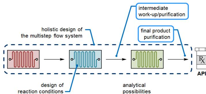
**Figure 2.1.** Hidden traps in the realization of multistep flow synthesis of APIs and the two types of purification based on their position.<sup>[2]</sup>
