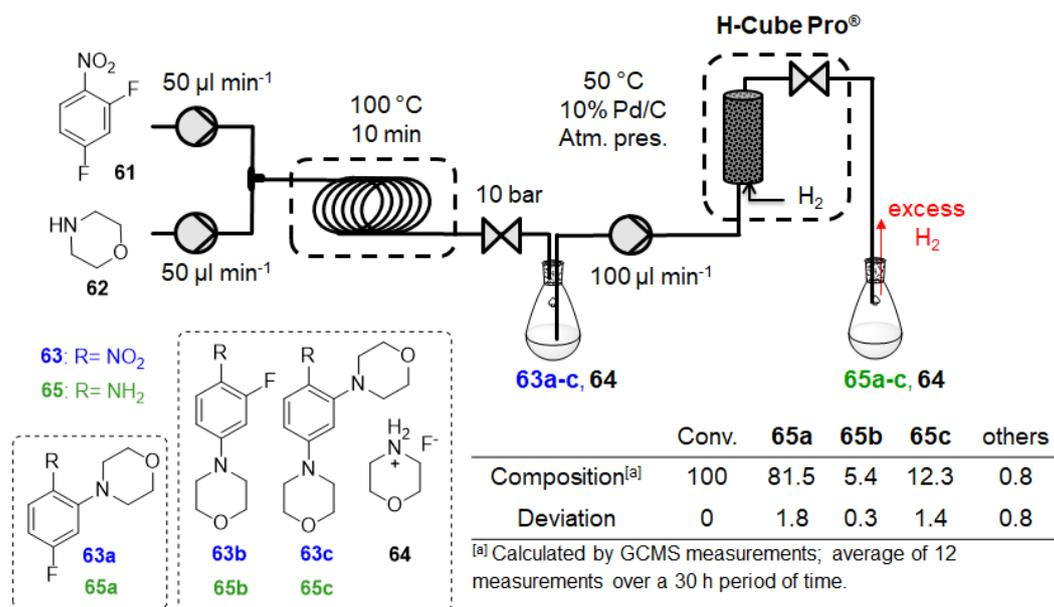
**Figure 3.4.** Continuous-flow  $S_NAr$  reaction of 2,4-difluoronitrobenzene (**61**) with morpholine (**62**) followed by a heterogeneous continuous hydrogenation of the nitro compounds (**63a-c**) to the corresponding anilines (**65a-c**), using a loop reactor and the H-Cube Pro<sup>TM</sup> device.
