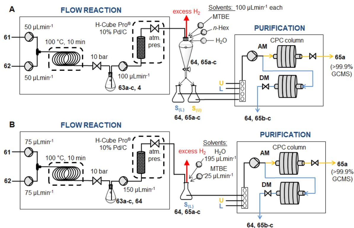
**Figure 3.5.** Flow chart of the two-step synthesis followed by a quasi-continuous MDM CPC purification, using: **A**, two-phase sample intake or **B**, one-phase sample intake. U: Upper phase of the chosen BLS, L: Lower phase of the chosen BLS;  $S_{(L)}$ : Sample solution in lower phase,  $S_{(U)}$ : Sample solution in upper phase.
