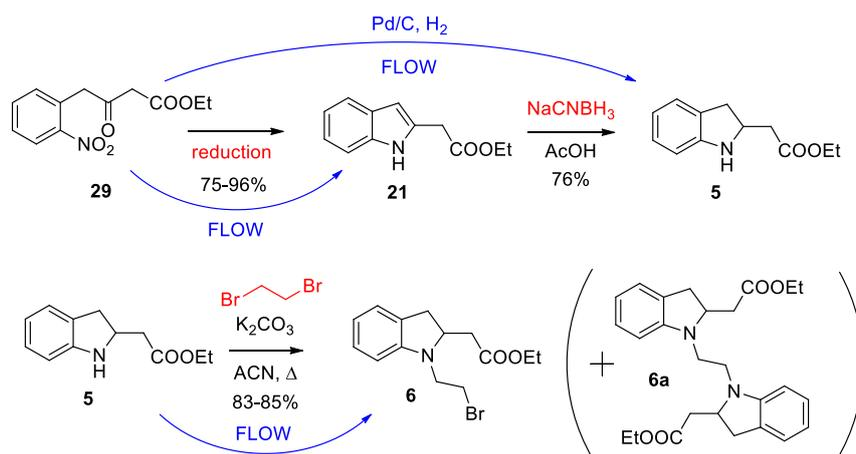
**Figure 3.2.** Application of flow chemistry in the synthesis of the intermediates of **2**.
