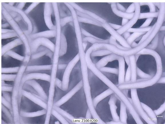
**Fig. 2** Digital optical micrograph of PHB fibers produced by wet spinning at 0.08 ml/min spinning rate.
