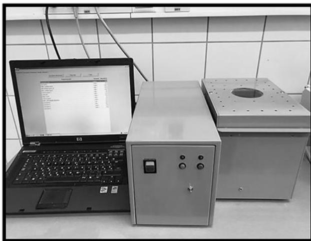
1. Figure: Prototype of self-developed laboratorial bread making instrument
