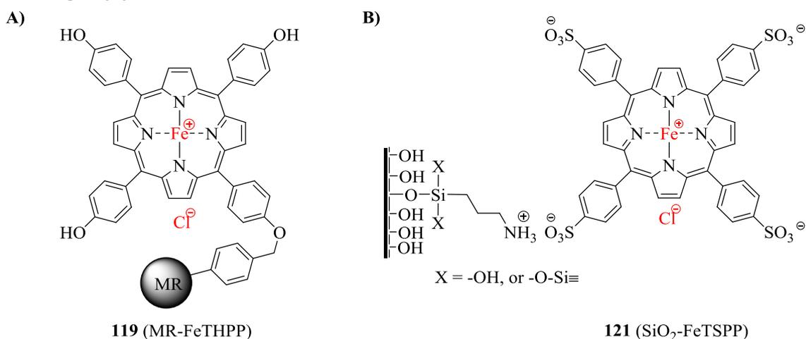
**Figure 4.** Structure of A) **119** *Merrifield-resin*- and B) **121** 3-aminopropyl-functionalized silica supported porphyrin catalysts.
