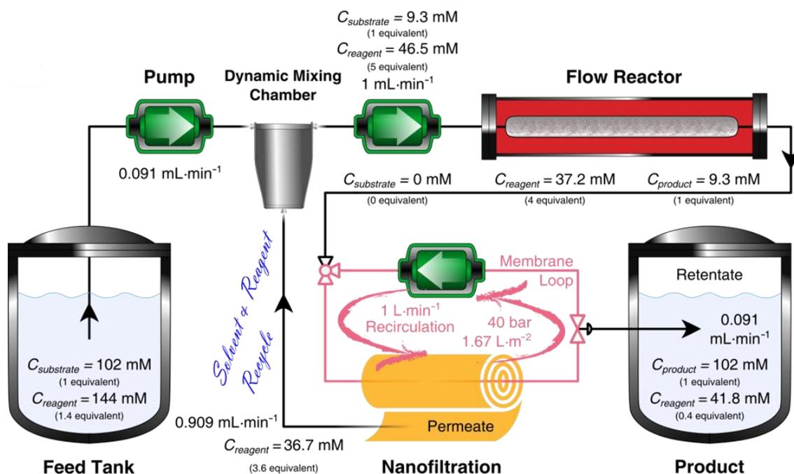
**Figure 1.** Experimental setup of the hybrid system applying solvent and excess of reagent recycle.
