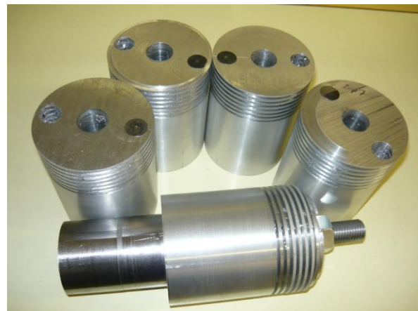
Fig. 4.10 b – Photo of the specimens, prepared for orthogonal cutting
