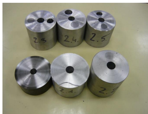
Fig. 4.02 b – Photo of the specimens, used for the cross turning
