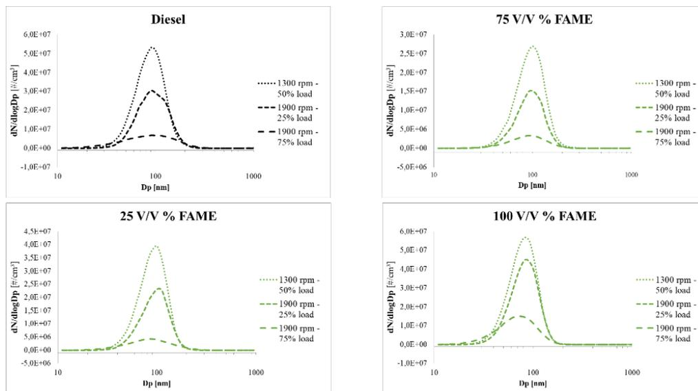
**4. Figure Thesis 3.b.** – Particulate emission of the engine in range of 10 nm – 1000 nm of electrical mobility diameter
