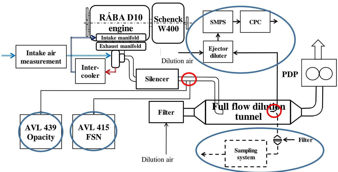
**Figure 2.** Experimental set up for measuring the particulate relevant emission of the engine
