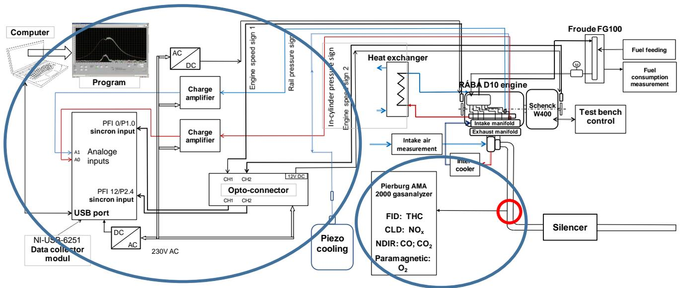
**Figure 1.** Experimental set up for indicating and for measuring the gaseous pollutants of the engine
