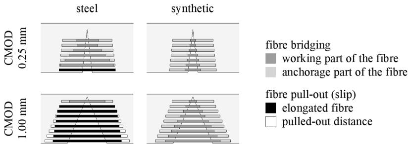
**Figure 7.** Fibre bridging and fibre pull-out of steel and synthetic fibres
