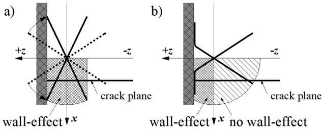
**Figure 5.** The impact of wall-effect on the quantity of fibres intersecting the cross section in the case of a) steel fibres and b) synthetic fibres
