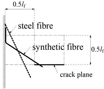
**Figure 4.** Over-reaching of steel and synthetic fibres to the adjacent cross section zone when the wall-effect is active
