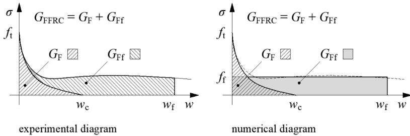
**Figure 8.** Experimental and numerical diagram of fibre reinforced concrete
