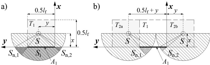
**Figure 3.** a) Interpretation of fibres intersecting the face  $A_1$  from space  $T_1$  b) Penetration from the adjacent spaces  $T_{2a}$  and  $T_{2b}$
