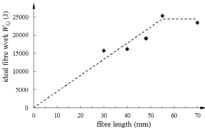
**Figure 10.** Fibre length and fibre-work correlation
