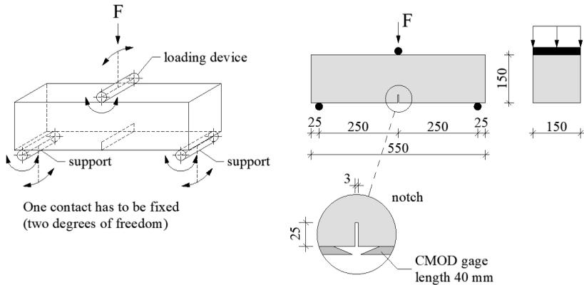
**Figure 1.** Three point bending beam test according to the recommendation of RILEM TC 162
