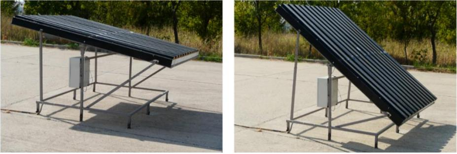
Figure 5: TSC measurement setup used for the complex energy evaluation
