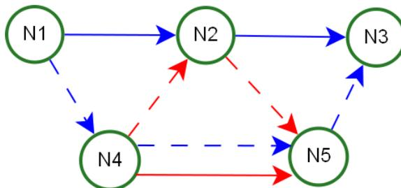
Figure 4: Behaviour of the ratio of the length of the backup path and the primary path. Primary paths are drawn by solid lines, while backup paths by dashed lines. Length of every edge is 1.
