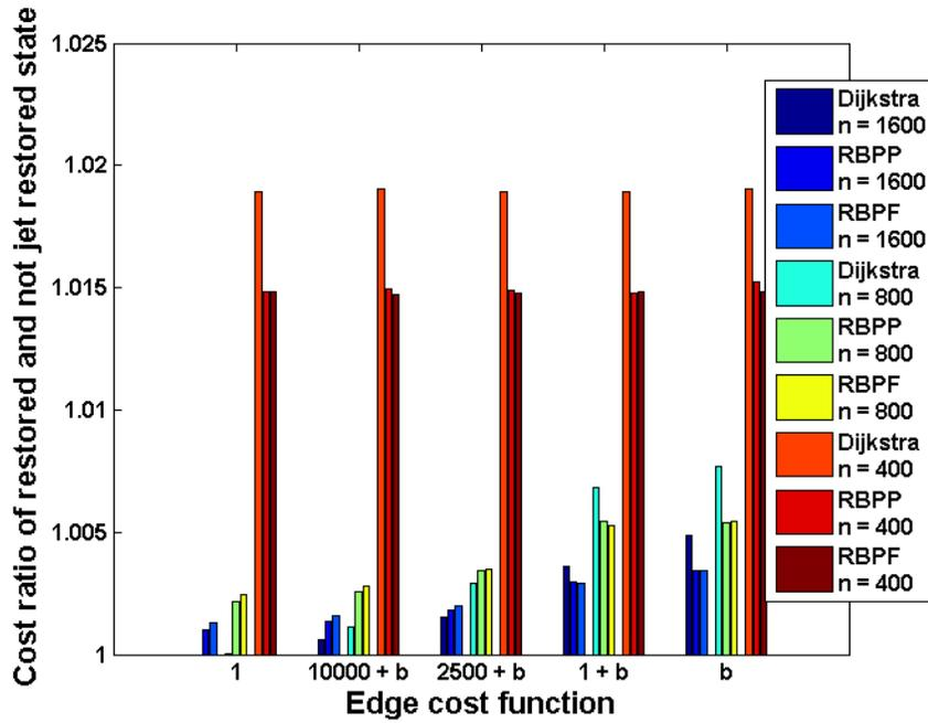
(a) Ratio of the routing cost before and after the restoration
