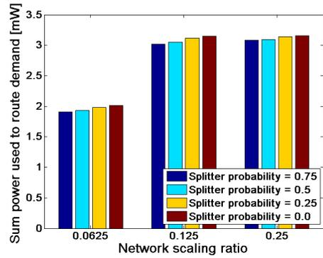
(b) Total power load of the network if output power cannot be fine tuned for every direction at optical splitters
