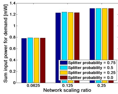
(c) Total used demand power if output power can be fine tuned for every direction at optical splitters
