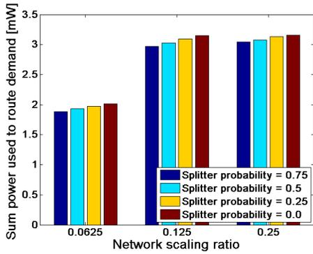
(a) Total power load of the network if output power can be fine tuned for every direction at optical splitters
