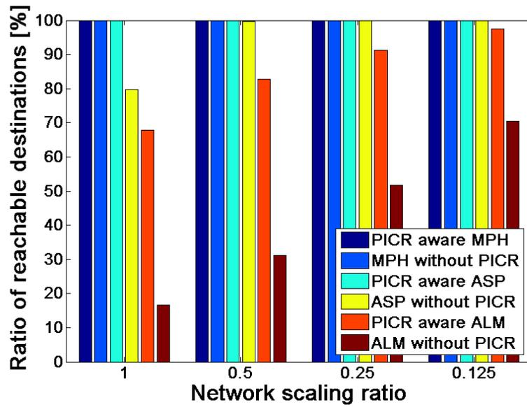
Figure 6: Ratio of the routable demands with the newly proposed algorithms and without it
