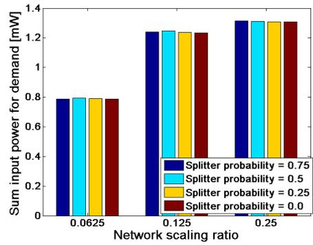
(d) Total used demand power if output power cannot be fine tuned for every direction at optical splitters
