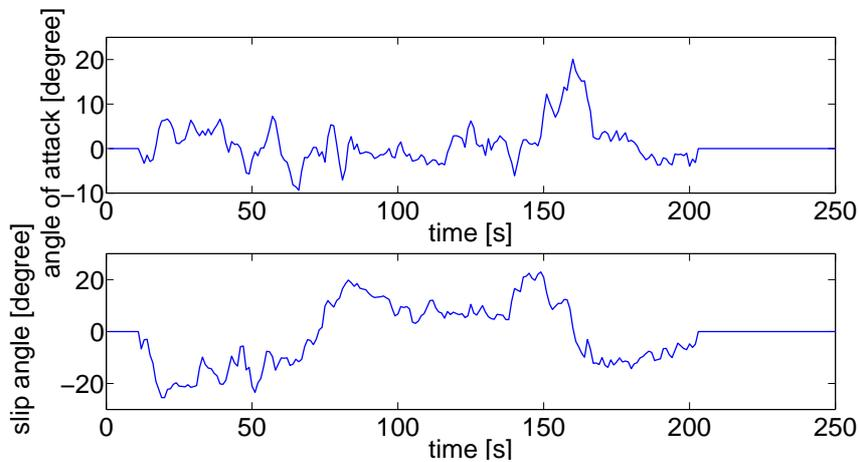
Figure 6: Angle of attack and side slip angle calculated from the 3D orientation
