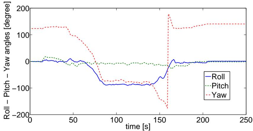
Figure 5: RPY angles during the sail-plane flight
