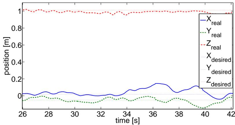
Figure 3: Helicopter position during position hold
