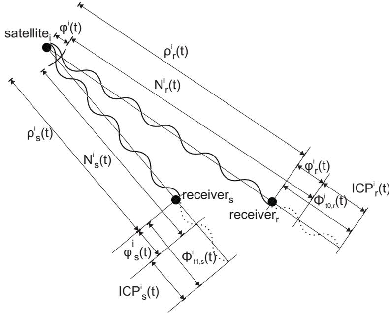
Figure 2: Structure of the carrier phase differential GPS
