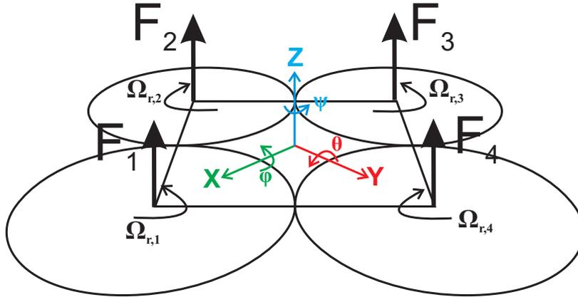
Figure 1: The structure of the quadrotor helicopter
