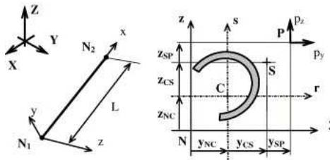
Fig. 3 Beam element local systems and eccentricities
