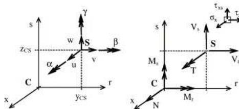
Fig. 4 Local displacement parameters and stress resultants
