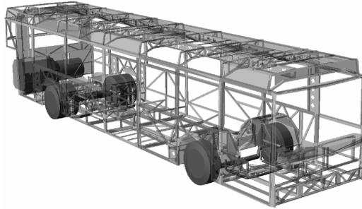
Fig. 1 Integral bus body under frame
