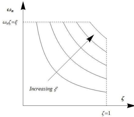
Fig. 6 Frequency vs. damping ratio for different damping coefficient
