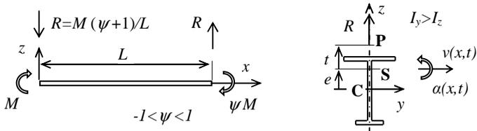
Fig. 5 Displacement, Rotations and coordinates system (sample cross section)
