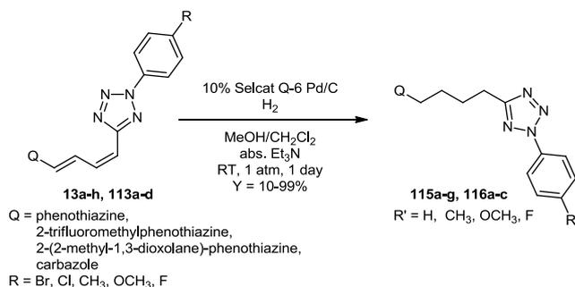
**Scheme 6.** Catalytic hydrogenation of *N*-dienylphenothiazines and -carbazoles
