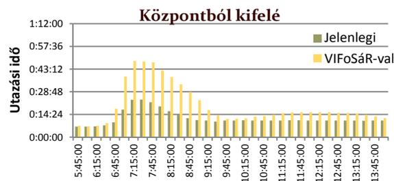
**Fig. 5** Average travel times on the outbound lanes in different departure times
