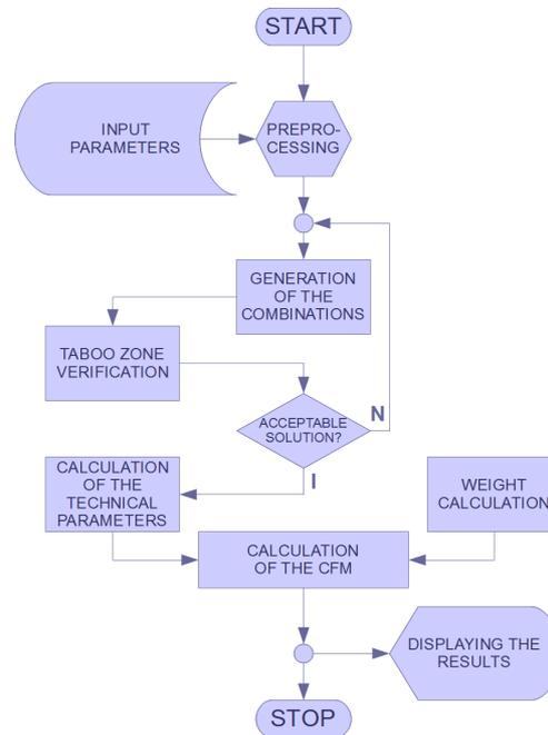
Fig.2: Project workflow in the design for configurations
