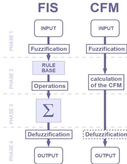
Fig.1: Comparison of the the FIS and the CFM method
