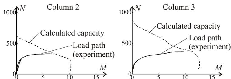
**Figure 11:** Comparison of the calculated load paths and the calculated capacity diagrams for GFRP confined columns.
