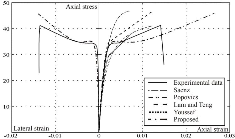
Figure 8: Comparison of the experimental results and the calculated  $\sigma(\epsilon)$  diagrams.
