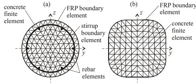
**Figure 6:** The finite element mesh of a circular cross-section with reinforcement (a) and rectangular cross-section (b).
