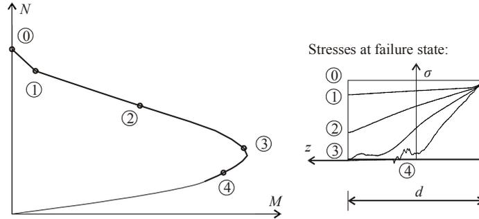
**Figure 14:** Average stress curves at failure.
