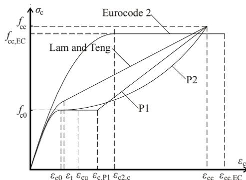
**Figure 15:** Stress-strain diagrams for simplified design.
