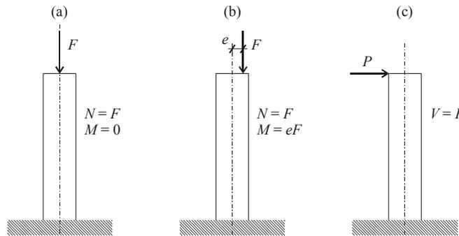
**Figure 1:** Typical loads on a column: concentric compression (a), eccentric compression (b) and horizontal load (c).
