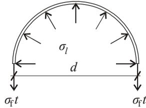
**Figure 2:** Confined circular cross-section.
