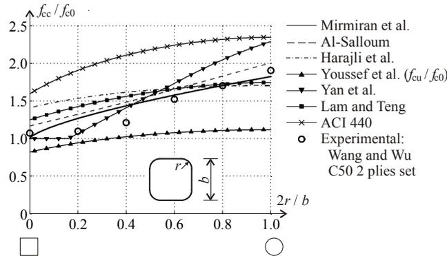
Figure 4: Effect of rounding of the edges on the ratio of confined strength ( $f_{cc}$ ) to unconfined strength ( $f_{c0}$ ) for square sections.
