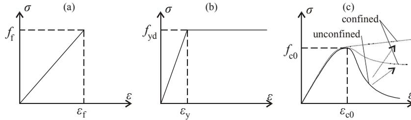
**Figure 5:** Typical stress-strain diagrams for the materials used in the model: FRP confinement (a), steel (b) and concrete (c).
