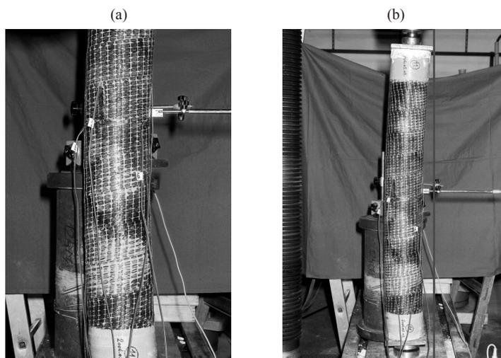
**Figure 10:** Instrumentation of specimen 11 (a) and the specimen curved due to the load (b).
