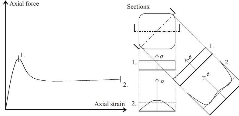
**Figure 20:** Axial stresses in rectangular cross-sections ( $f_{c0}$  is indicated by dashed lines).
