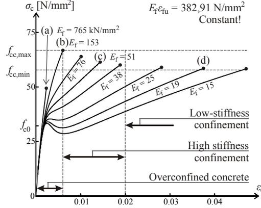
**Figure 13:** Effect of the stiffness of confinement on the stress-strain diagram of C30 concrete.
