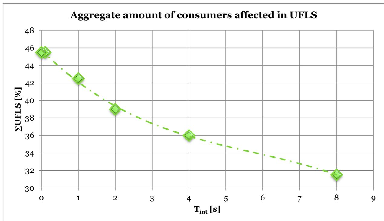
**Figure 2.: Aggregate amount of consumers affected in UFLS in function of integration time constant**
