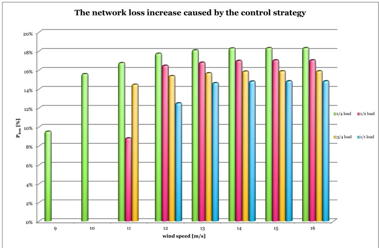
**Figure 3.:** The reachable network loss increases in % at different load profiles in function of wind speed
