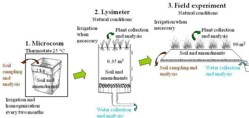
**Figure 1: Scaled-up technological experiments**
