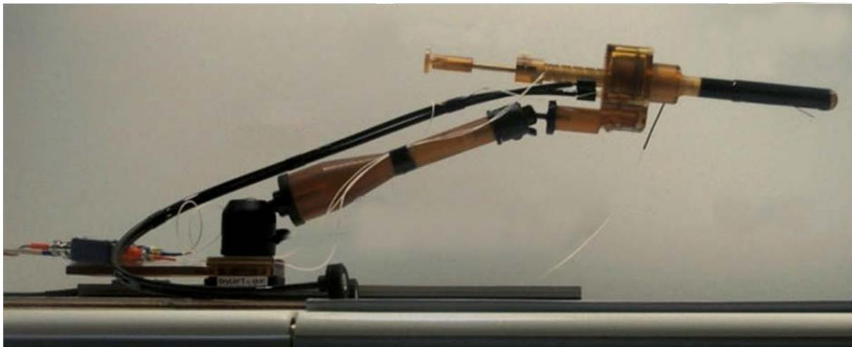
**Figure 2. Side view of the MRI-compatible intra-prostatic needle placement device developed by Krieger et al. (Source: [Krieger2005])**
