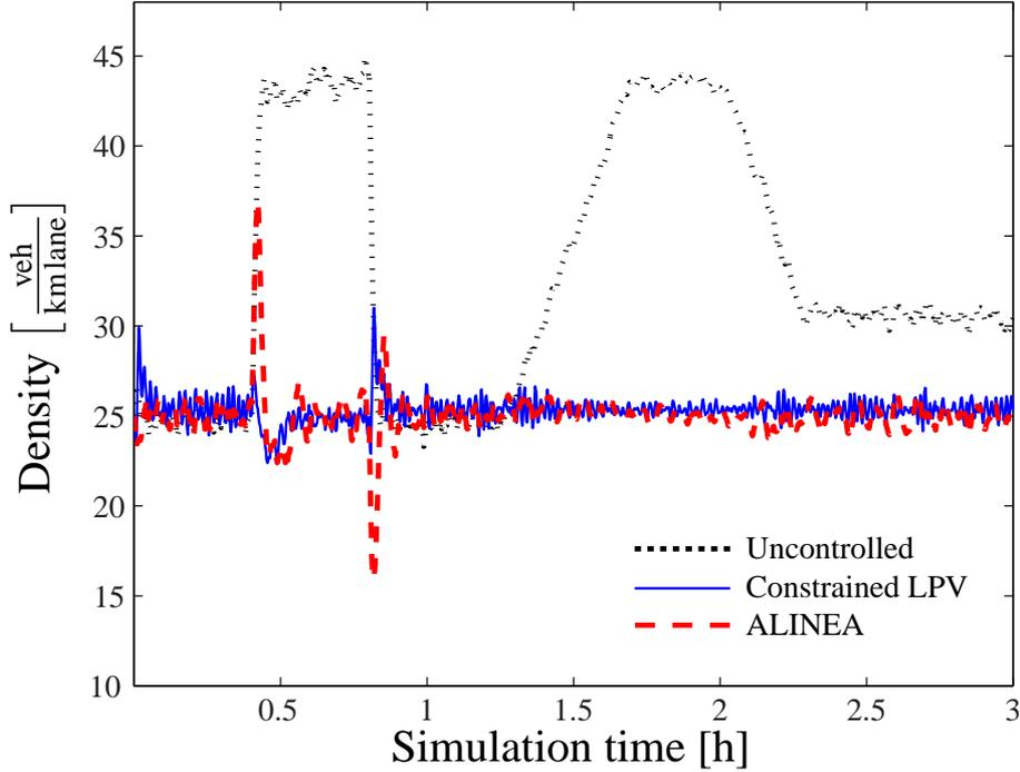
Figure 3: Comparison of the density evolution for the uncontrolled, polytopic controlled and the ALINEA controlled cases
