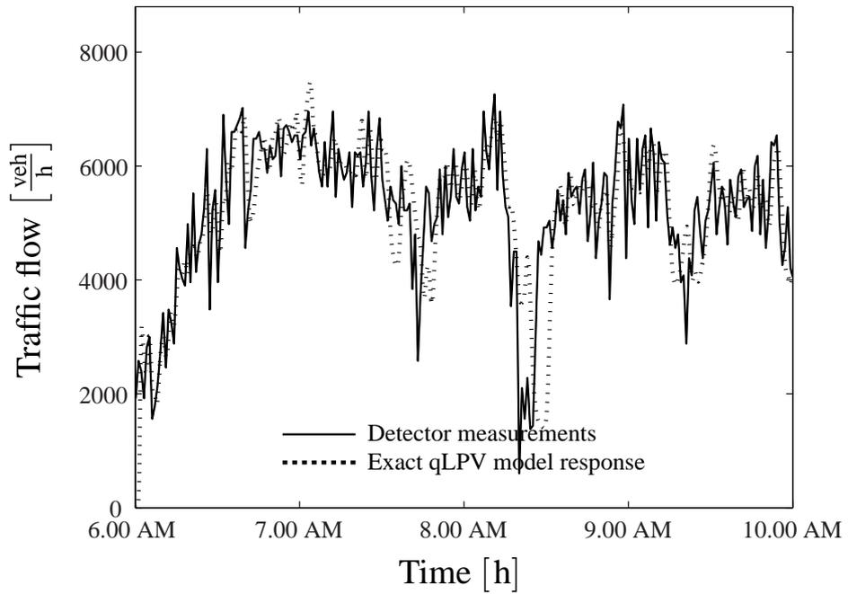
Figure 1: Comparison of exact qLPV speed and flow responses with detector measurements
