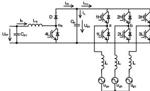
Figure 6, Main circuit arrangement for DLF control
