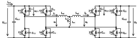
Figure 10. Main circuit arrangement of bidirectional galvanic isolated ZVS resonant DC/DC converter
