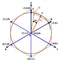
Figure 7, Voltage vectors of a voltage source inverter
