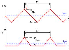
Figure 2, Current waveforms of continuous (upper) and discontinuous conduction
