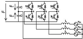
Figure 3. Simplified main circuit arrangement of three phase 3P+N type grid connected IGBT inverter
