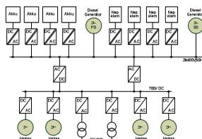
Figure 8. Main circuit diagram of the Green Yacht
