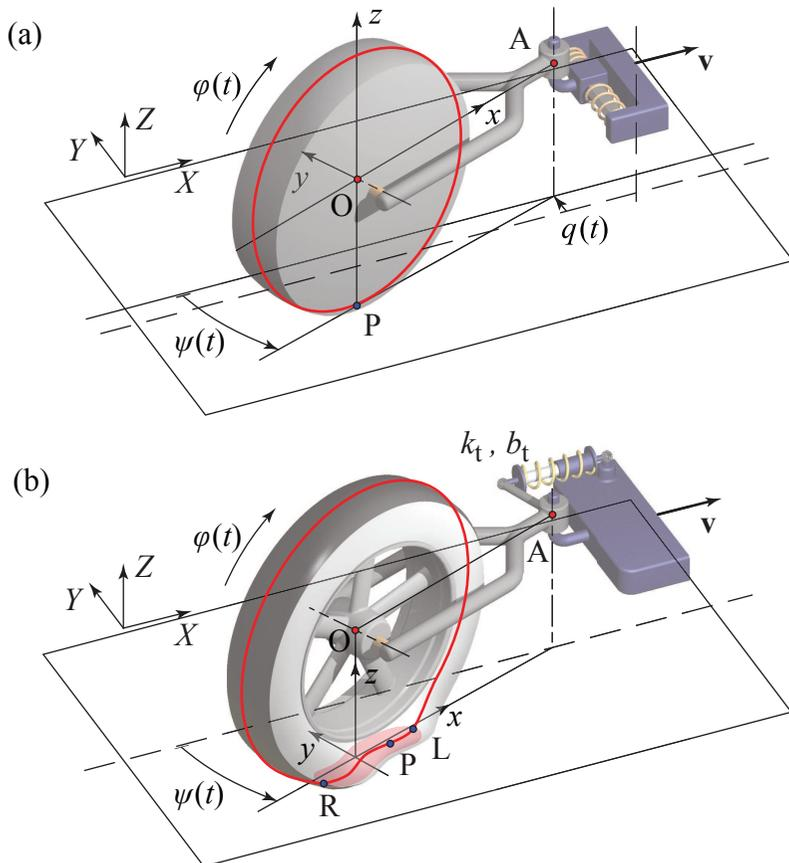
**Figure 1** Mechanical models: (a) single contact point model, (b) elastic tyre model.
