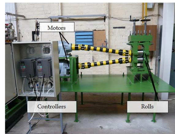
**Figure 3:** The rolling mill
