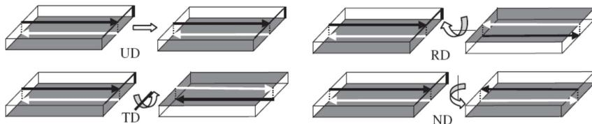
**Figure 2:** Different deformation routes of the differential speed rolling
