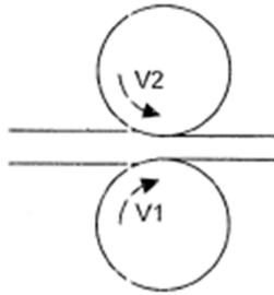
**Figure 1:** The technique of the differential speed rolling
