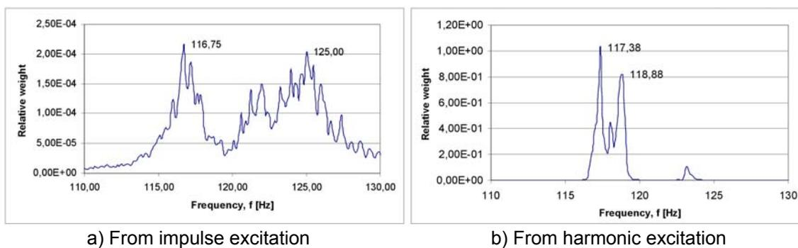
**Fig. 2.6** Average frequency spectrums with significant multiple peak around  $f_2$  (state 4 of P1)
