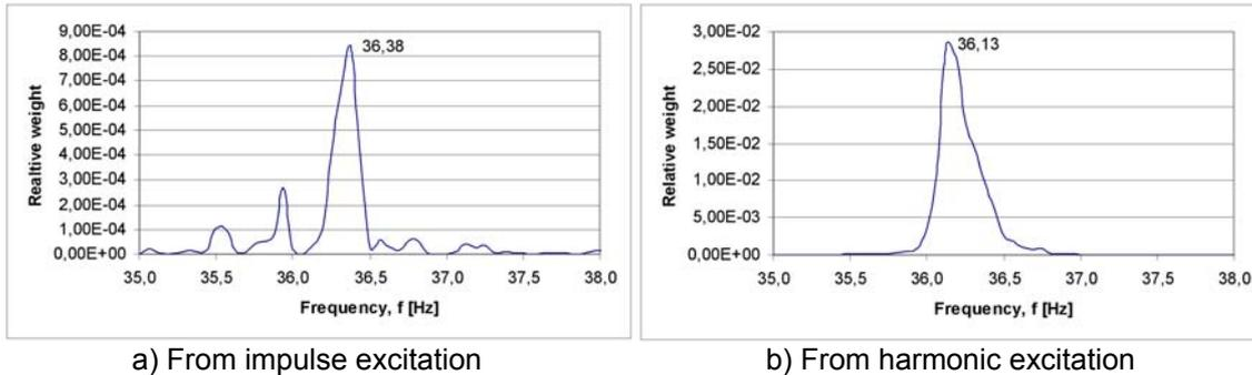
**Fig. 2.5** Average frequency spectrums for the first natural frequency ( $f_1$ ) (state 0 of P1)
