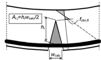
Fig.2.7 Assumed section of an individual crack
