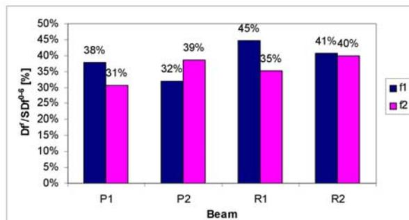
Fig. 2.12  $\Delta f$  [%] at the appearance of first cracks
