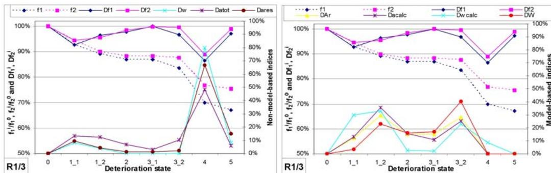
Fig. 2.9 Comparison of non-model-based and model-based indices for the R1/3 beam
