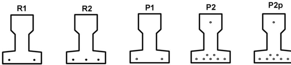
Fig. 2.1 Cross sections of model beams
