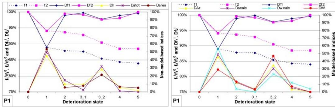
Fig. 2.10 Natural frequency shifts versus damage indices for the P1 beam
