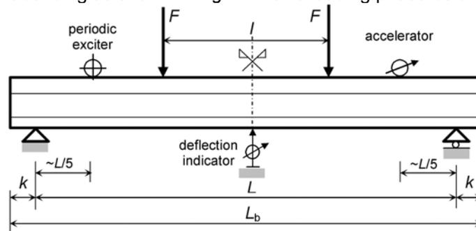
Fig. 2.4 Arrangement of beams under four-point bending
