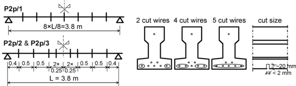
Fig. 2.2 Wire cuts for the P2p specimens
