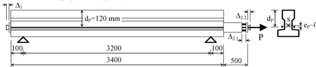
Fig. 2.3 Arrangement and geometry of post-tensioning for the P1 specimen
