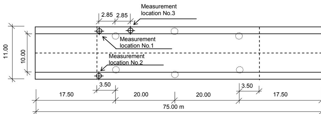
Fig. 2.15 Scheme of the investigated bridge and the measurement locations
